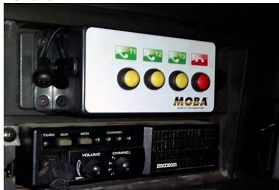
*The audiosystem allows drivers and dispatch centre to communicate with each other*
